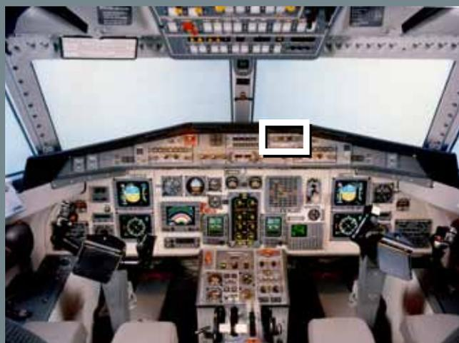
Above: typical J41 flight deck with the Reversionary Switch Panel highlighted.
