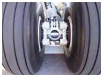
deflection. There are different tyre deflection values and maximum tyre rolling speeds with values of either, 32%, 35% or 36% deflection being used. The higher deflection values result in a flatter tyre which in turn causes a greater footprint and so greater friction thus requiring higher take-off speeds.
