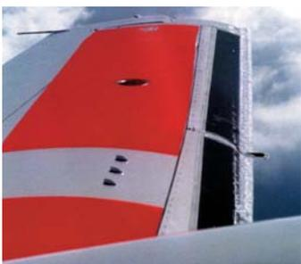
Above: ice accretion on a J41 wing following a simulated failure of the airframe de-icing boots
