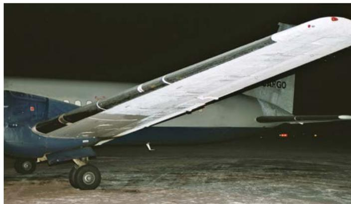
**Above and inset: turboprop operators need to be aware of icing conditions that may cause heavy accretion which could exceed the capabilities of the ice protection systems**
