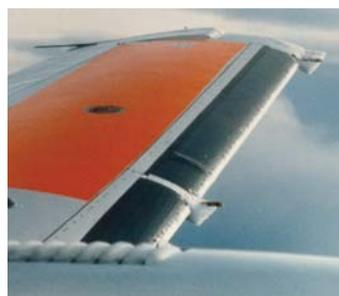
Above: ice accretion on a J41 wing during normal operation of the airframe de-icing boots
